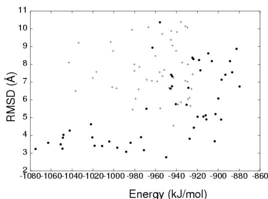
Fig. 1. Plots of the energy and RMSD values of low energy conformations obtained from CSA search using the initial and the refined parameters for the protein 2GB1. The crosses and the filled circles denote the results obtained using the parameters before the optimization and after the 6-th iteration, respectively.
